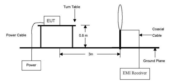
The diagram below shows the test setup that is utilized to make the measurements for emission from 30 Mb to 1 Mb Emissions.
