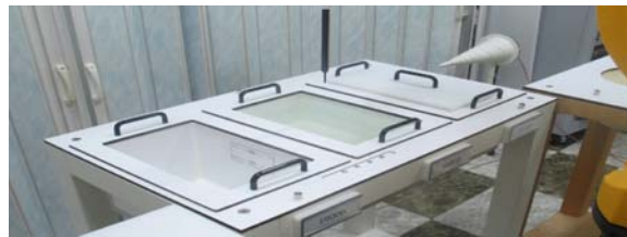
Figure 3.6 Modular Flat Phantom
