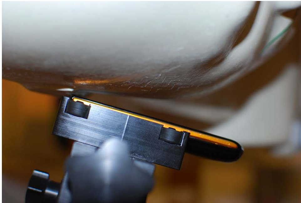
Figure 19-2 SAR Test Setup Photo 2
