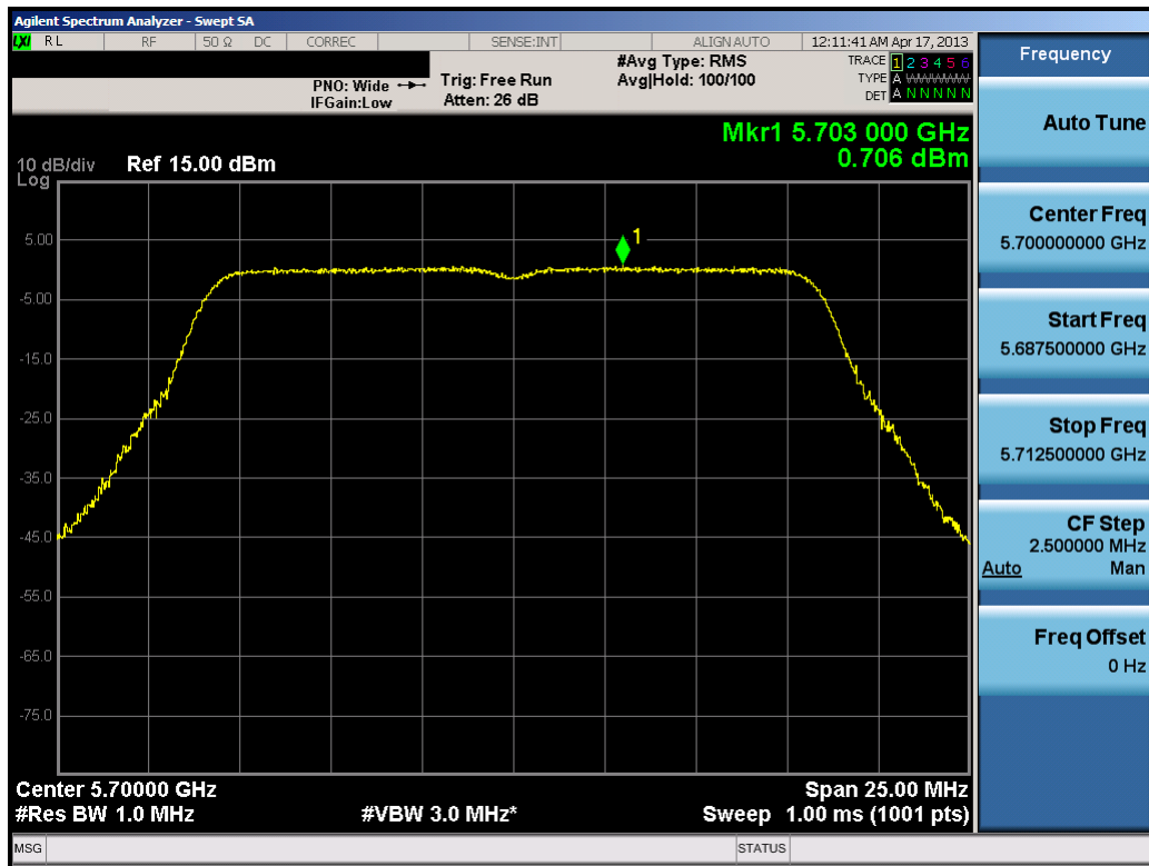
Plot 6-53. Peak Power Spectral Density Plot (20MHz BW 802.11n (UNII Band 3) – Ch. 140)
