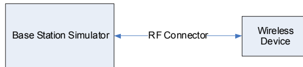
Figure 9-2 Power Measurement Setup
