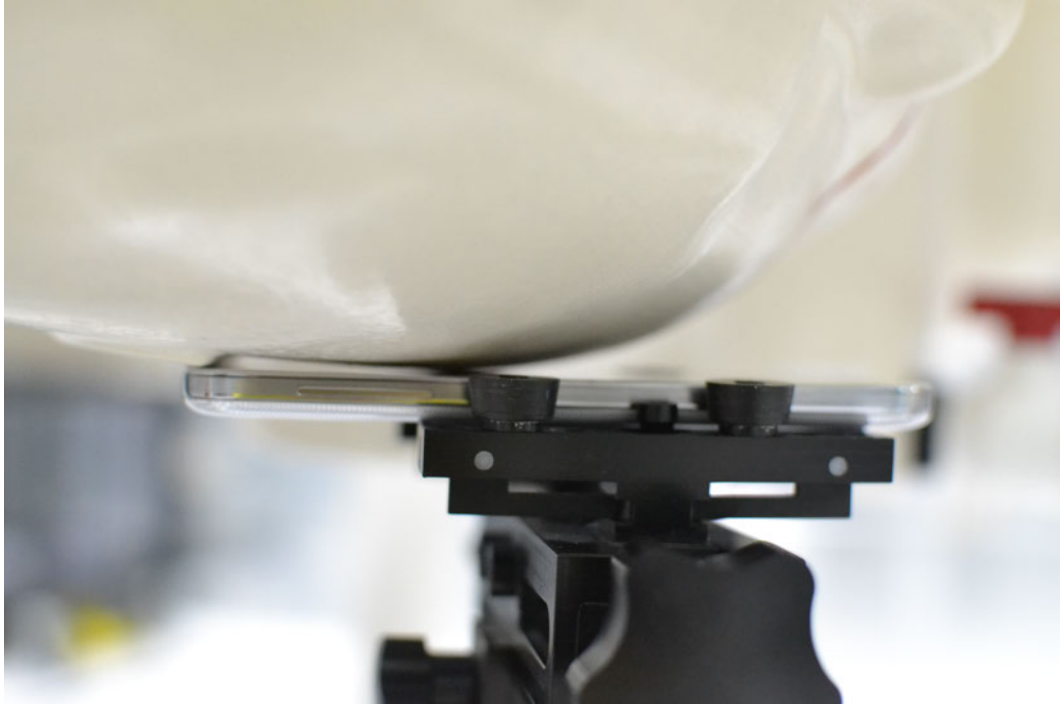
SAR Test Setup Photo 1: Right Cheek
