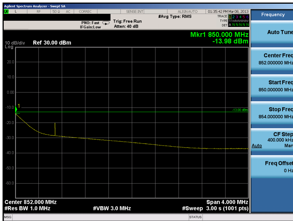
Plot 7-21. 4MHz Span Plot (Cellular WCDMA Mode – Ch. 4233)
