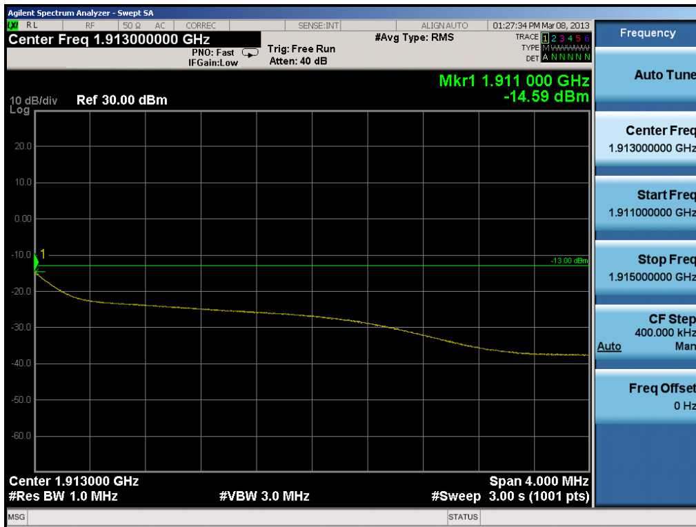
Plot 7-33. 4MHz Span Plot (PCS WCDMA Mode – Ch. 9538)
