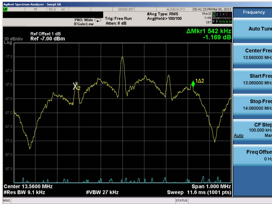
Figure 8-2. 20dB Bandwidth Plot
