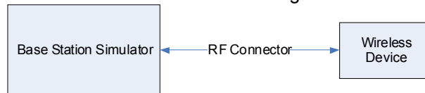
Figure 10-1 Power Measurement Setup
