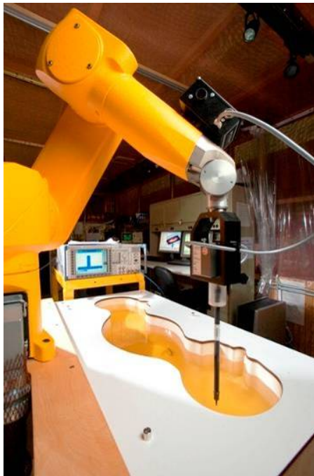
Figure 3-2 SAR Measurement System
