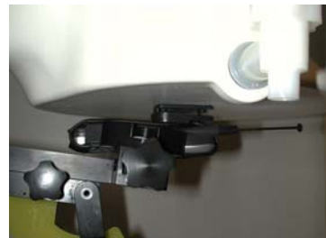
Fig 9-5 Body SAR Sample Photo (Not Actual EUT)
