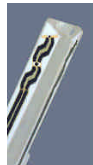
Figure 3.2 Probe Thick-Film Technique
