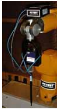
Figure 5-7 SPEAG Robotic System
