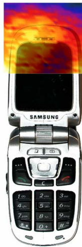
Figure 28 Sample H-field Scan Overlay
