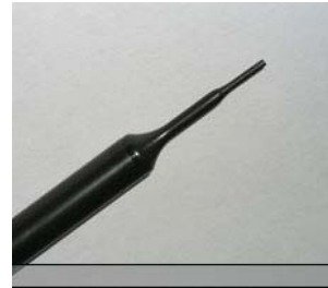
Figure 3.4 Probe Thick-Film Technique
