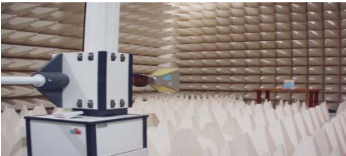
Figure2. Photograph of 3m Fully Anechoic Chamber
