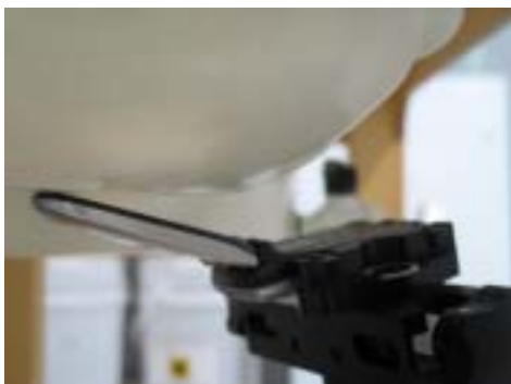
Figure 8.3 Right Head SAR Test Setup -- Ear/Tilt 15° Position--
