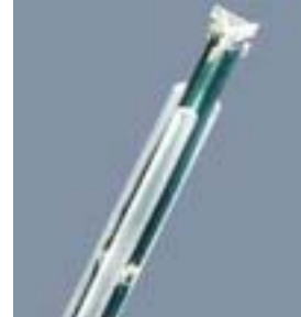
Figure 3.4 Probe Thick-Film Technique
