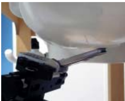
Figure 8.5 Left Head SAR Test Setup -- Ear/Tilt 15° Position--
