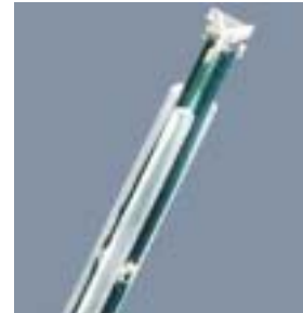
Figure 3.4 Probe Thick-Film Technique
