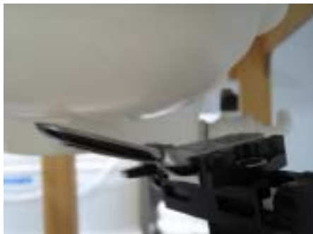
Figure 8.7 Right Head SAR Test Setup -- Ear/Tilt 15° Position--
