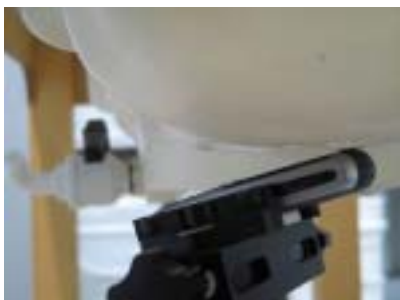
Figure 8.5 Left Head SAR Test Setup -- Ear/Tilt 15° Position--
