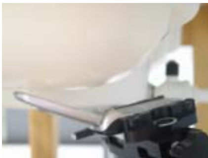
Figure 8.7 Right Head SAR Test Setup -- Ear/Tilt 15° Position--
