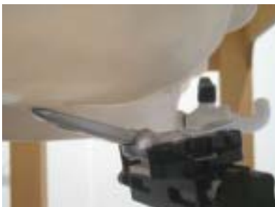
Figure 8.7 Right Head SAR Test Setup -- Ear/Tilt 15° Position--
