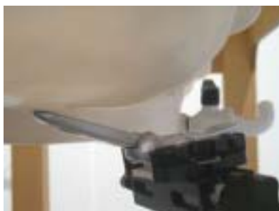
Figure 8.3 Right Head SAR Test Setup -- Ear/Tilt 15° Position--
