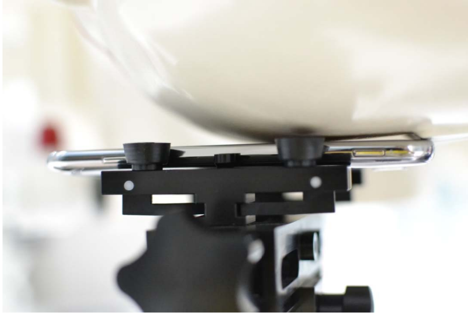
SAR Test Setup Photo 3 - Left Cheek
