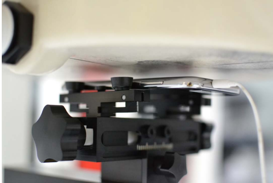
SAR Test Setup Photo 11 - Body at-Worn 1.0 cm
