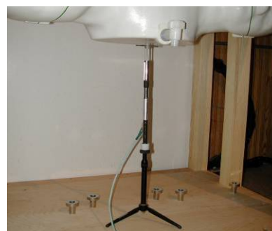
Figure 11-2 System Verification Setup Photo
