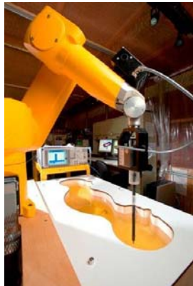
Figure 4-1 SAR Measurement System
