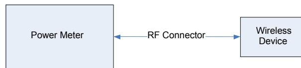
Figure 10-4 Power Measurement Setup
