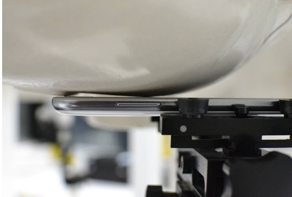
SAR Test Setup Photo 1 – Right Cheek
