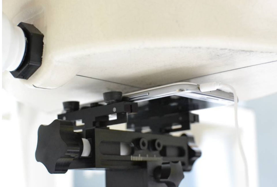
SAR Test Setup Photo 11 – Body-worn at 1.0 cm
