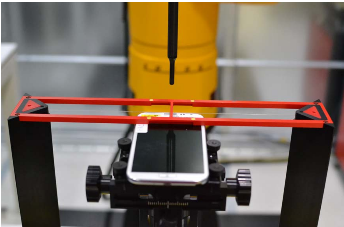
Figure 17-2 HAC Phantom Plane Alignment
