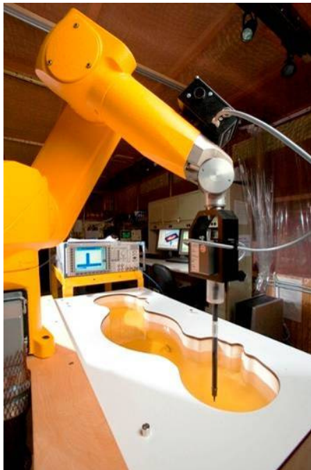
Figure 3-2 SAR Measurement System
