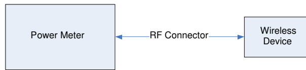
Figure 12-1 Power Measurement Setup
