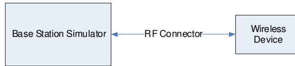
Figure 11-1 Power Measurement Setup
