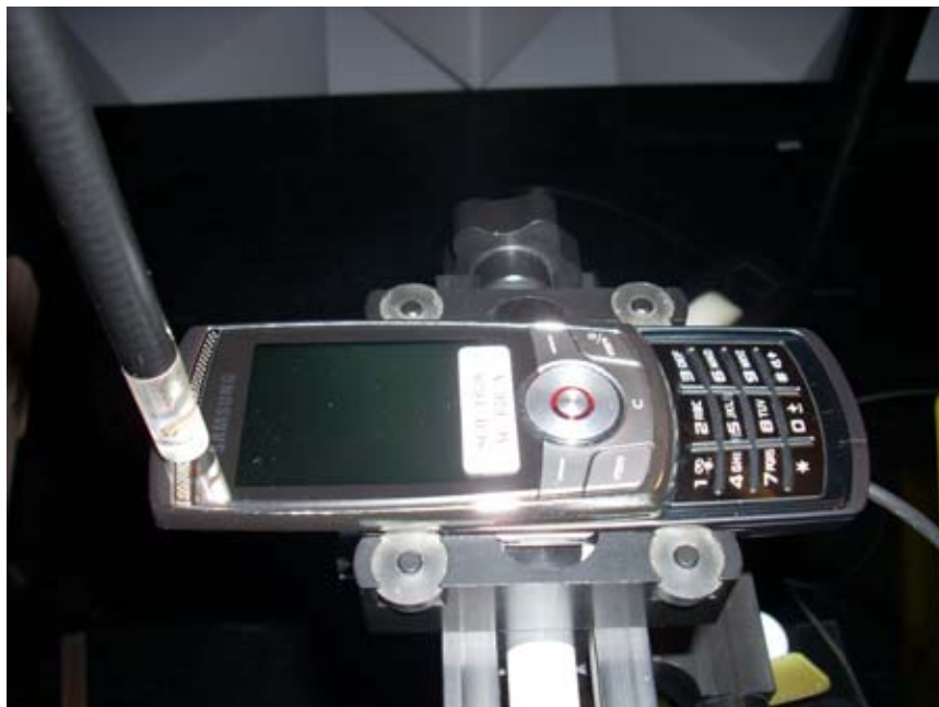
Figure 13-2 Test Setup for Wireless Device
