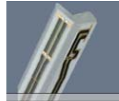
Figure 5-1 E-field Free-space Probe
