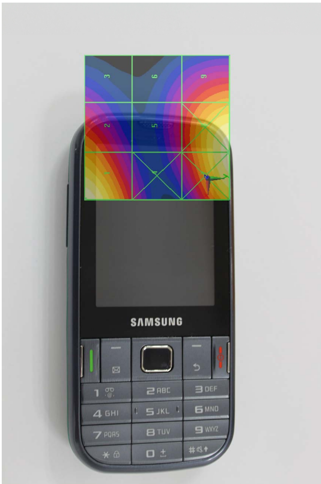
Scan overlay with actual device(E-field)
