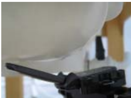
Figure 8.7 Right Head SAR Test Setup -- Ear/Tilt 15° Position--
