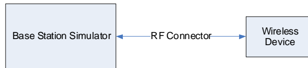
Figure 14-1 Power Measurement Setup
