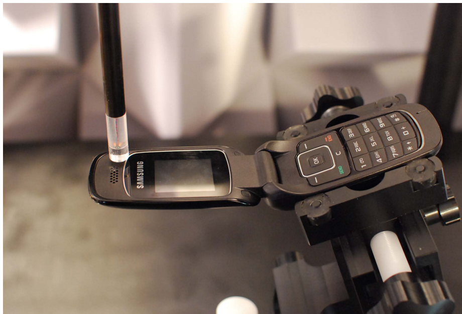
Figure 12-2 Test Setup for Wireless Device
