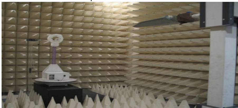
Figure2. Photograph of 3m Fully-Anechoic Chamber
