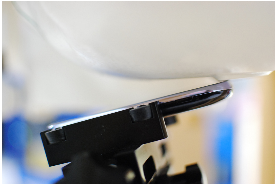
SAR Test Setup Photo 4 – Left Tilt
