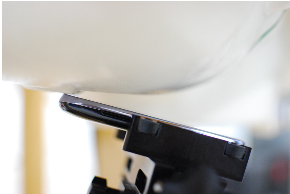
SAR Test Setup Photo 2 – Right Tilt
