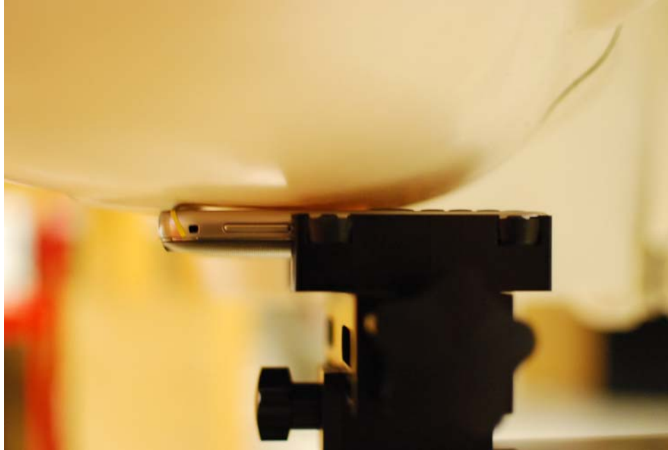
SAR Test Setup Photo 1: Right Touch
