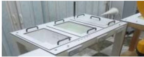
Figure 3.6 Modular Flat Phantom
