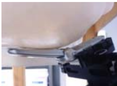
Figure 8.2 Right Head SAR Test Setup -- Cheek / Touch Position--
