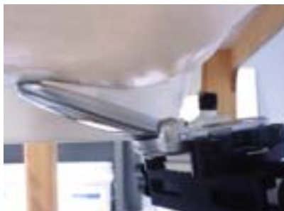
Figure 8.3 Right Head SAR Test Setup -- Ear/Tilt 15° Position--
