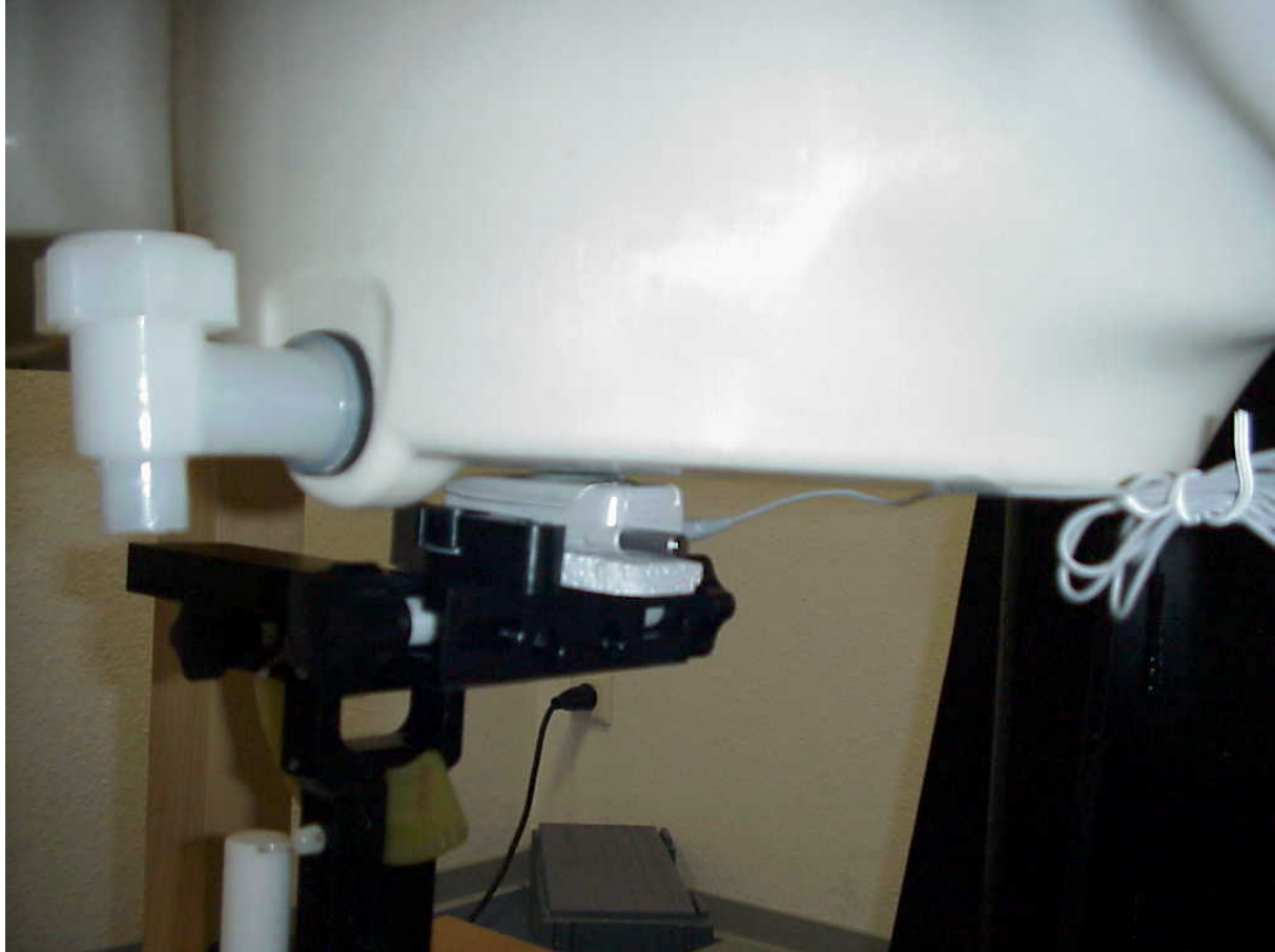
Photo 7: test position at the flat phantom, front side, test with headset
