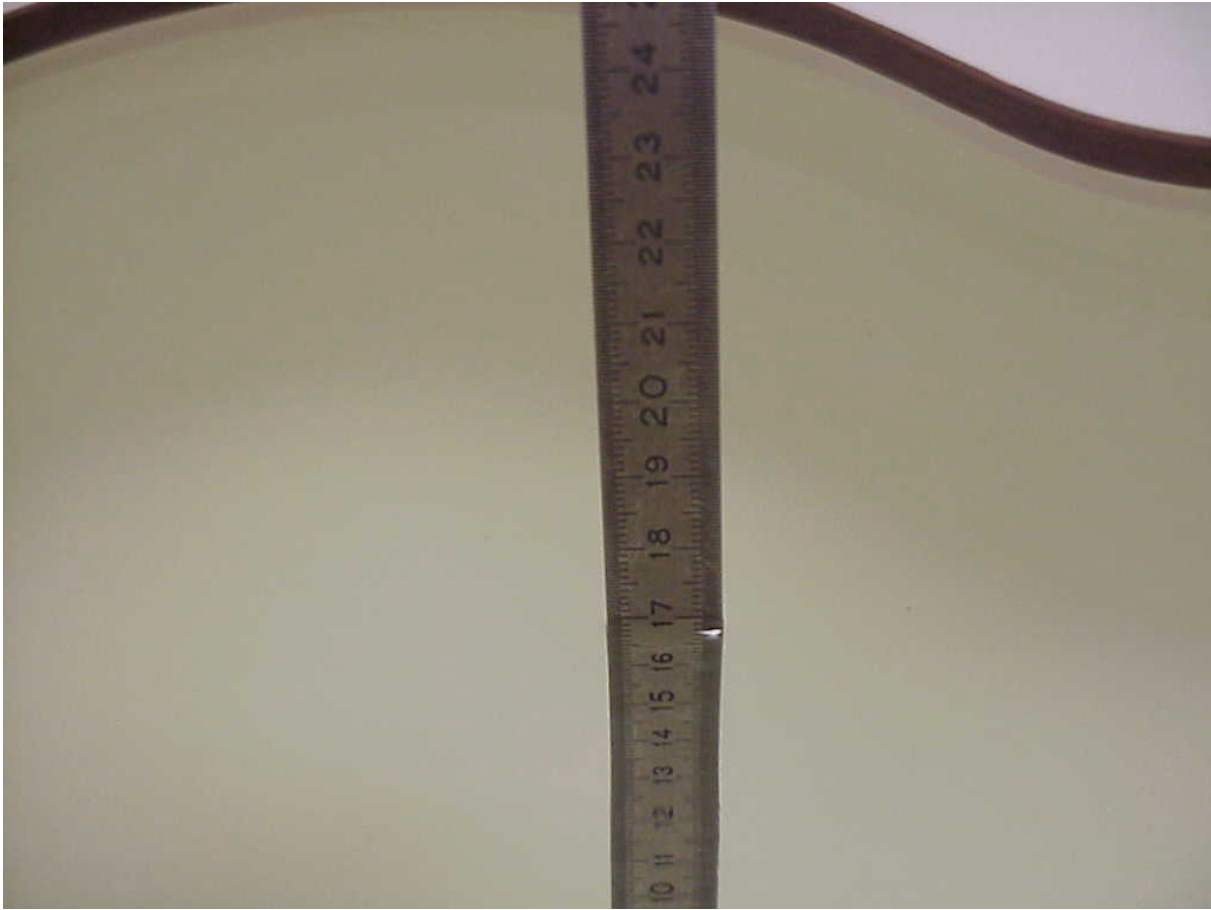
Photo 11: Liquid depth 1900 MHz head tissue simulation
