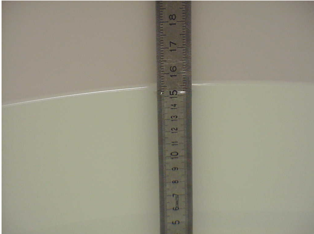
Photo 12: Liquid depth 1900 MHz body tissue simulation
