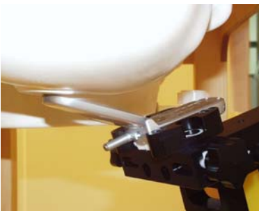
Figure 8.5 Right Head SAR Test Setup -- Ear/Tilt 15° Position--
