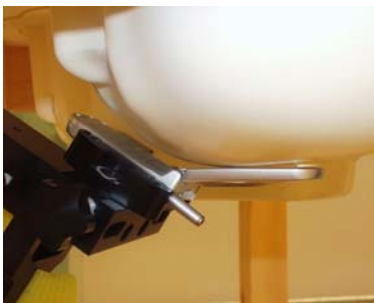
Figure 8.2 Left Head SAR Test Setup
