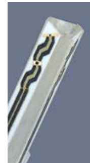
Figure 3.4 Probe Thick-Film Technique
