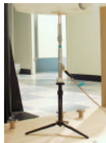
Figure 7.1 Dipole Validation Test Setup
