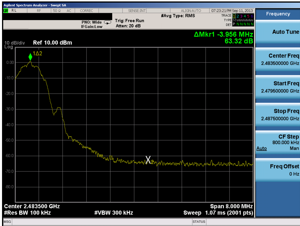
Plot 6-11. Band Edge Plot (Bluetooth (LE) – Ch. 39)
