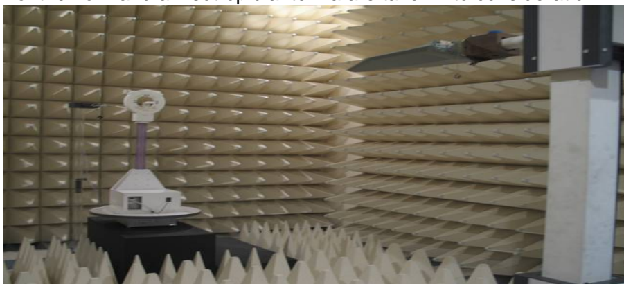
Figure2. Photograph of 3m Fully-Anechoic Chamber
