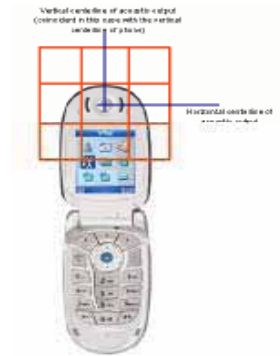
Figure 5.1 Wireless Device and Measurement Plane
