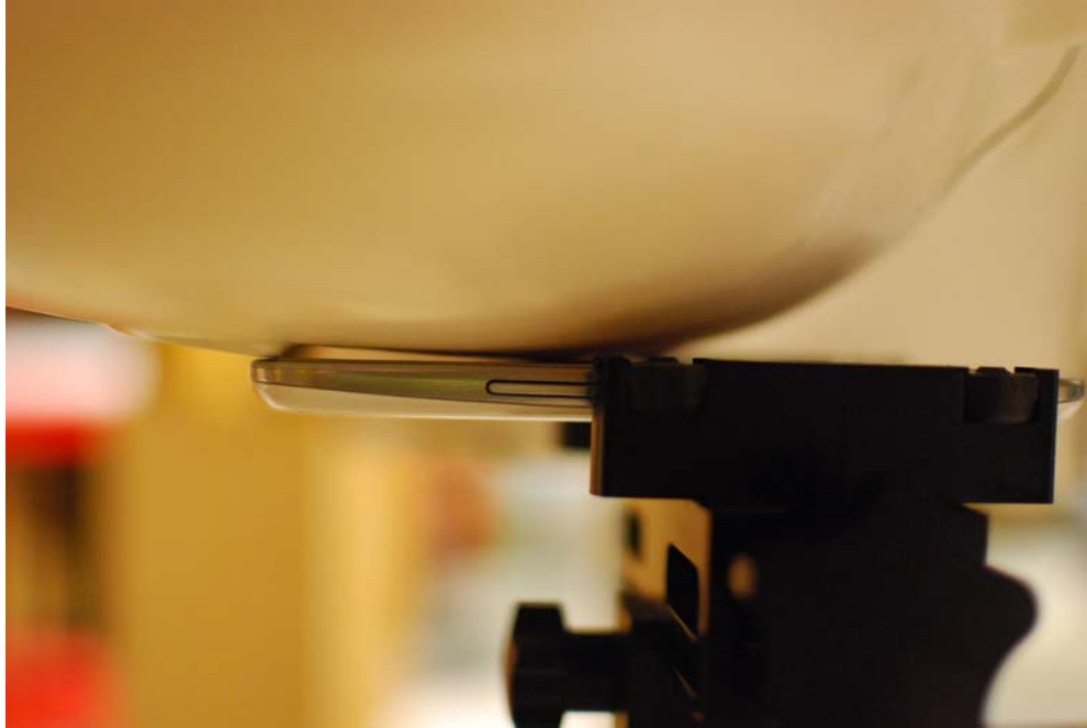
SAR Test Setup Photo 1: Right Touch
