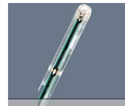
Figure 5-2 H-Field Free-space Probe
