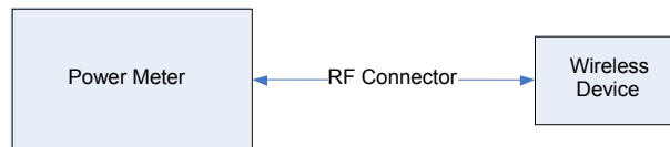
Figure 10-3 Power Measurement Setup
