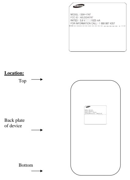
Label is placed inside of the battery compartment.
