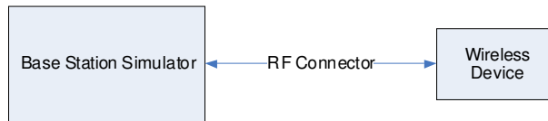
Figure 14-1 Power Measurement Setup
