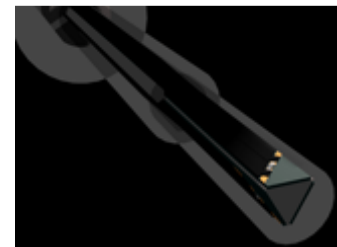
Figure 5-3 Triangular Probe Configuration
