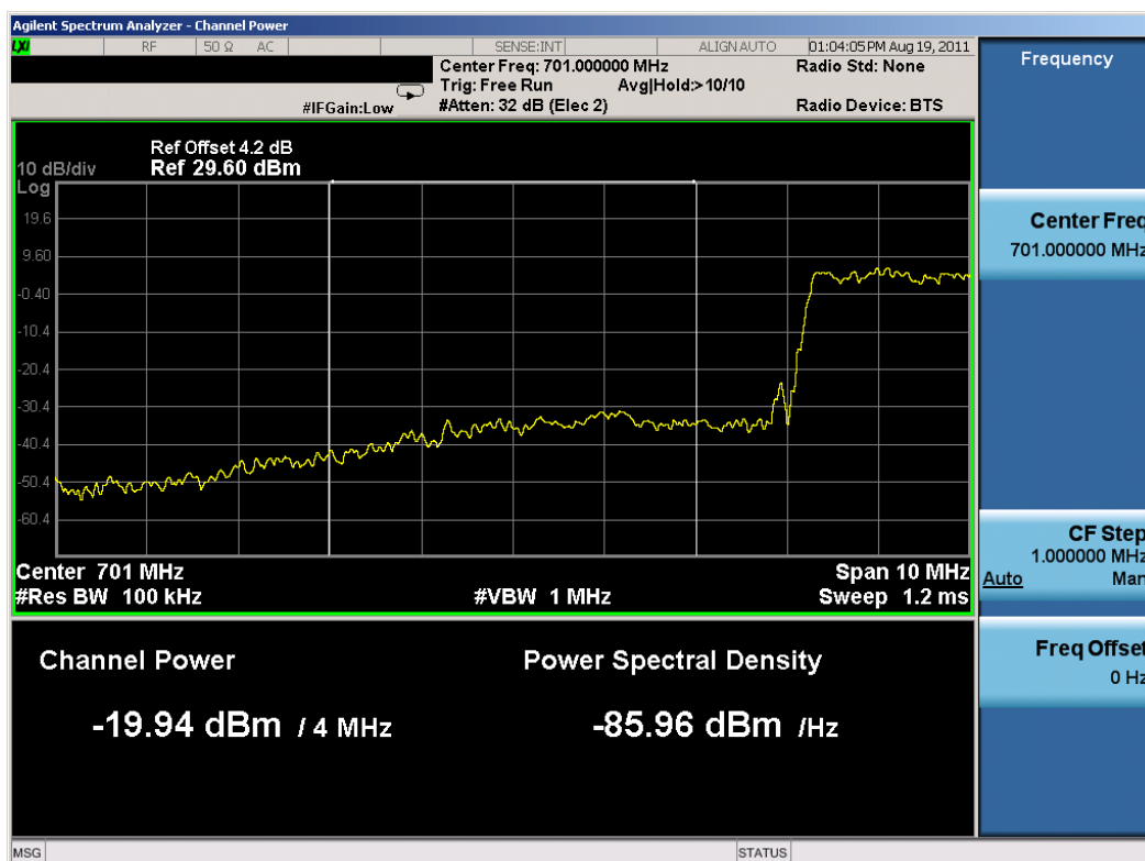
Plot 7-7. Extended Lower Band Edge Plot (5MHz BW, QPSK RB Size = 25, Offset = 0)
